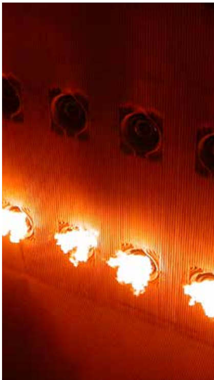
Oil Fired FyrStorm Igniters
